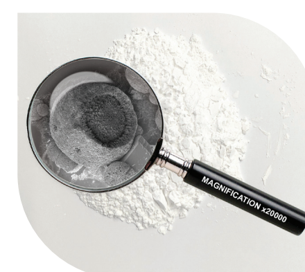
Scanning Electron Micrographs of PCC polymorphs obtained by Lixiviation & Carbonation route (Spheroidal Vaterite and Rhombohedral Calcite)
