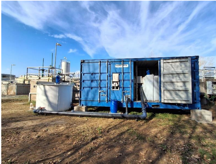
Rotating Belt Filter (RBF) pilot unit at the Sant Celoni Wastewater Treatment Plant (WWTP). Photo: Carla Vazquez Gomara / ACCIONA Agua
